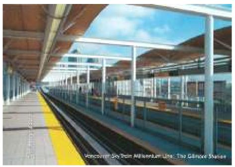
"We used Timberstrand on the Gilmore Station," Nielsen says. "It is really an engineered chipboard that comes in inch-and-a-half strips that can run as long as you want. We used a steel kingpost and a wire tensioner and that worked out really well. The panels were prefabricated in the shop and they could just be brought out on the site and dropped into place. They were preroofed so the membrane was already in place."
