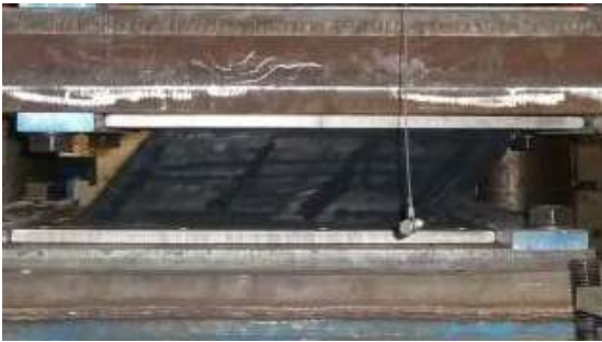
Fraser Heights Bridge – bearing shear / compression test.
